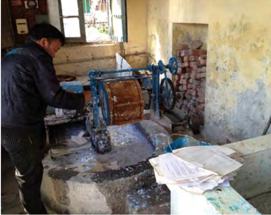
Figure 53 (a - h). Pictures of paper-making process that I took part in. The pulp this day is made from school assignments and scraps from a cotton t-shirt factory. These are common sources of raw material for their paper.
