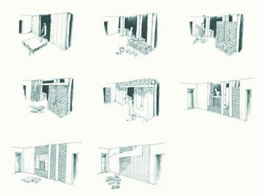
The construction process of the heating wall system
