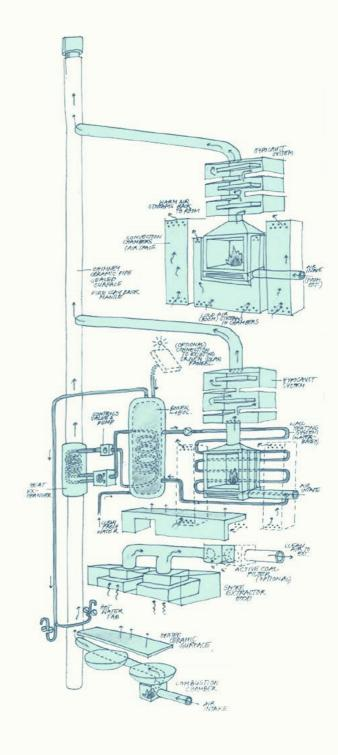
The heating wall system structure schema
