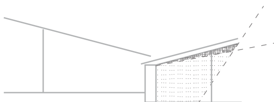
Scheme of solar angles (winter and summer), using the sun to heat the building and let enough light in Group 1: What a waste
