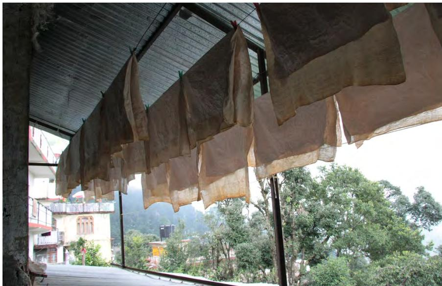
*Figure 53. Drying sheets of cleaned cotton to be used in papermaking.*
